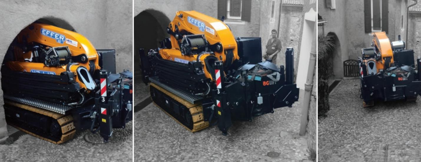
Less centimetres in height, length, width and a millimetric translation control, permit to the reach places previously inaccessible to other cranes with same performance. Noteworthy sites: 5070X1850, H 2615 mm.
